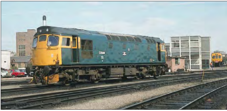
Above: for decades the staple diesel diet north of the border was the BRCW/Sulzer Type 2 Bo-Bos of classes 26 and 27. Of the latter type, 27 008 was captured on Haymarket depot on 16 April 1982.
