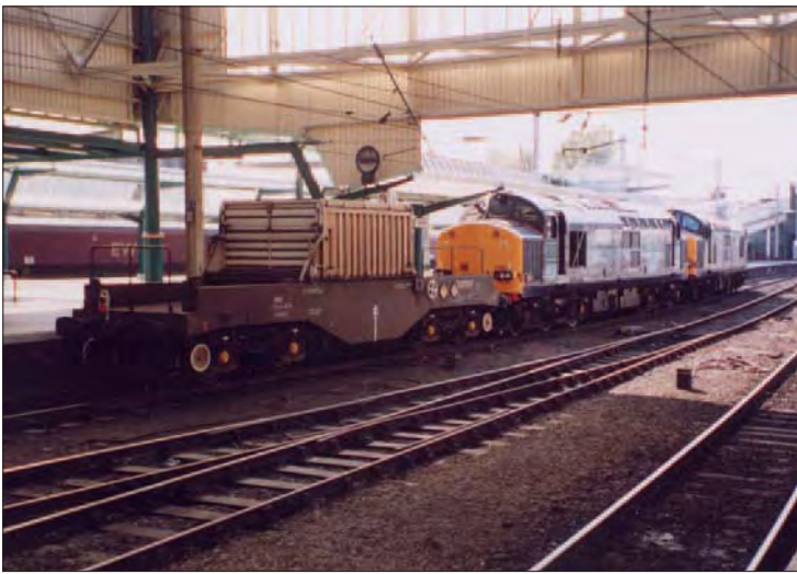
Above: a short train worth modelling – one TTA nuclear flask wagon is rolled through Carlisle by Direct Rail Services' Class 37s Nos.37 602 (leading) and 609 (trailing).
