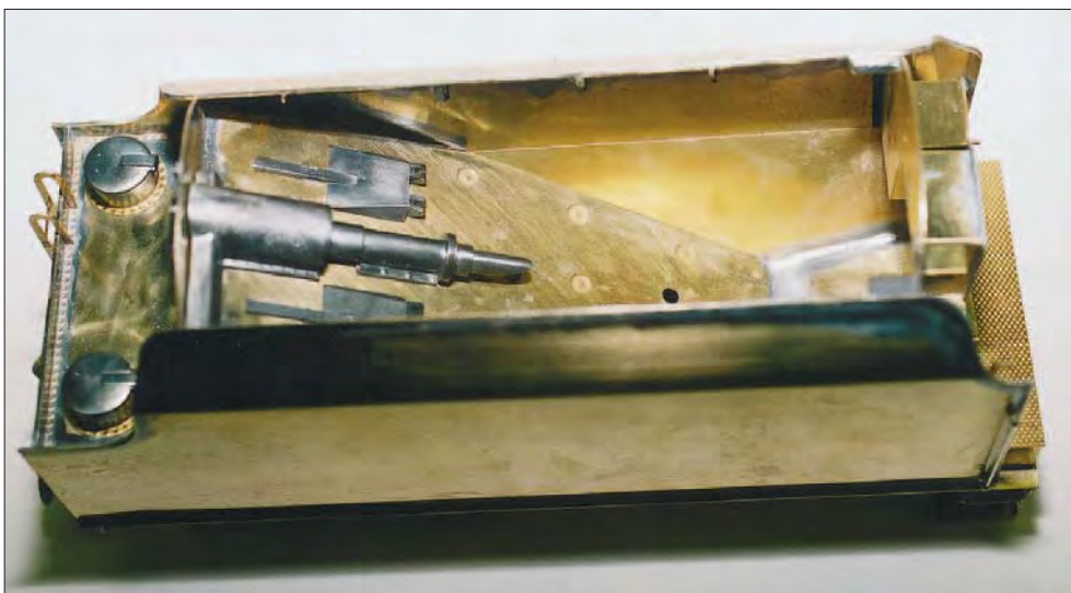
Left: the tender nearing completion. The coal pusher details are in white metal.
