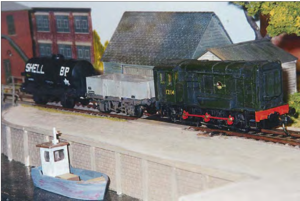
Left: a BR diesel shunter, converted from a Roco model by Chris Ellis, trundles down the riverside track. The steel open wagon has a scratchbuilt styrene body on a Lima under-frame. Plans are in LNER Wagons by Peter Tatlow, an invaluable source of research material.
