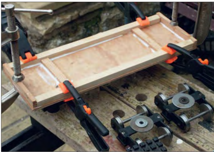
Above: flat wagon floor has solebars, buffer beams and cross timbers glued in place.
