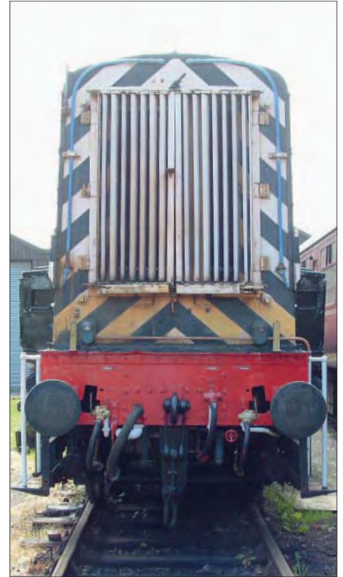
Above: 08 944 is the current dual-braked Class 08 available to the East Lancashire Railway Carriage & Wagon Department and this view dated 12 June 2004 of the nose shows how the model should look without the ladders. Note also the buffer beam pipework associated with air and vacuum braking.
