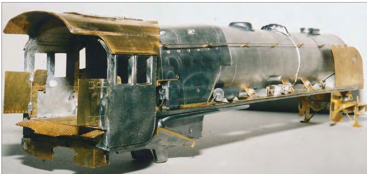
Below: rear view of the body. The backhead has not yet been fitted.
